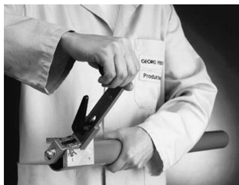
Chamfering the pipe
