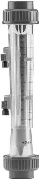
The limit contact serves to monitor externally the limited flow values and can be adjusted to any flow value on the corresponding scale. The magnet built into the float closes or opens a reed contact in the limit contact. This is a bistable switching function because the switching status remains when the float is taken from the contact.
